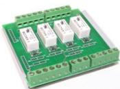
**ICR-44 - Intercom Relay Module 4X4** - Tech Works makes a variety of intercom Relay modules for routing audio and calls in signals. The ICR-44 is a snap track mount 4 relay assembly designed to allow multiple master audio routing by a PLC.
